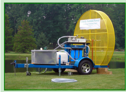
GP210 Mobile Water Treatment Facility
